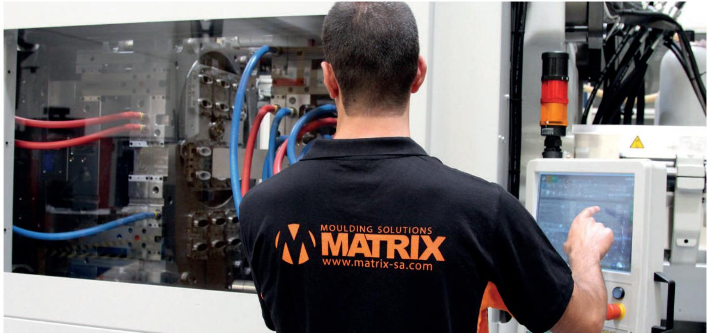
The trials area allows us to thoroughly **check** all the **injection parameters** and work **cycles** that have been agreed with the customer.
